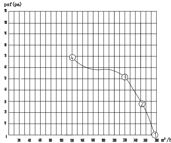
PS: Fan working performance tested with Meer wall plate, and under standard atmospheric pressure at 20 °C.
